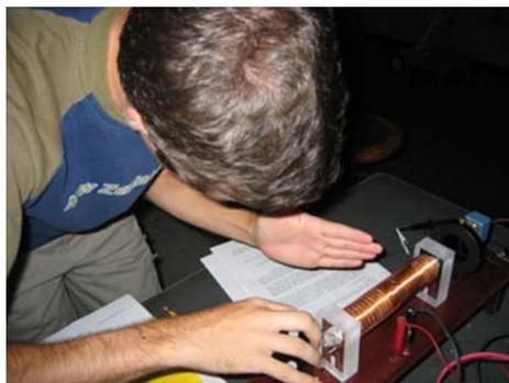
A fine adjustment of the Faraday rotation apparatus.
