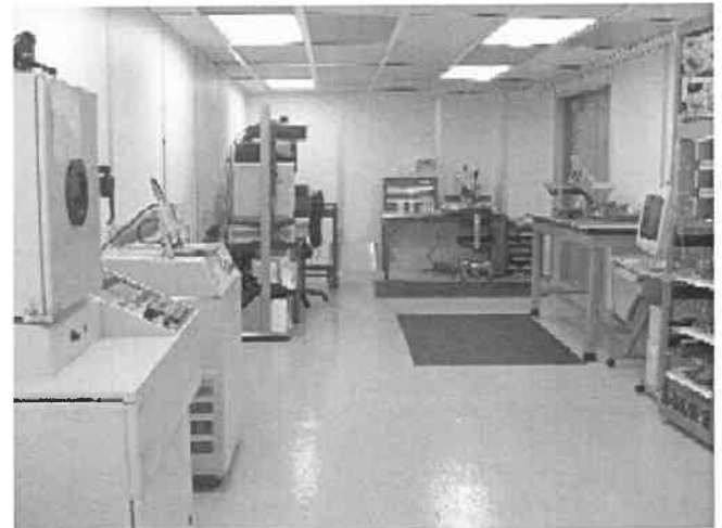
New class 1000 clean room. Not seen in the figure is an even more controlled class 100 clean room with entry from the class 1000 room. This facility was largely funded by a DOE grant of the high-energy group, with additional Department, College and University support. The facility is now used by both the high energy and condensed matter groups.
