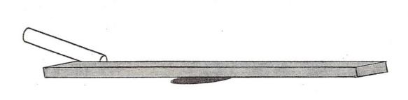
Balance the wooden 2" x 4" on the inverted watchglass. Stroke the PVC pipe against a piece of neoprene (or the hard rubber rod against the fur) and hold it near the end of the 2x4. The force will be large enough that you can rotate the 2x4.
