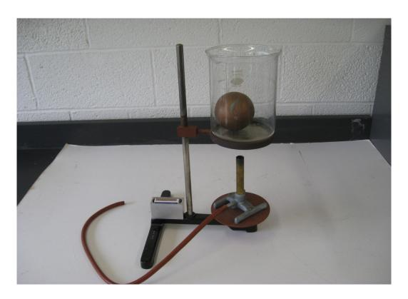
Use special, hollow, copper ball the weight of which has been so adjusted that the ball will float in cold water (below roughly 20 °C) and sink in hot water (above roughly 50°C).
