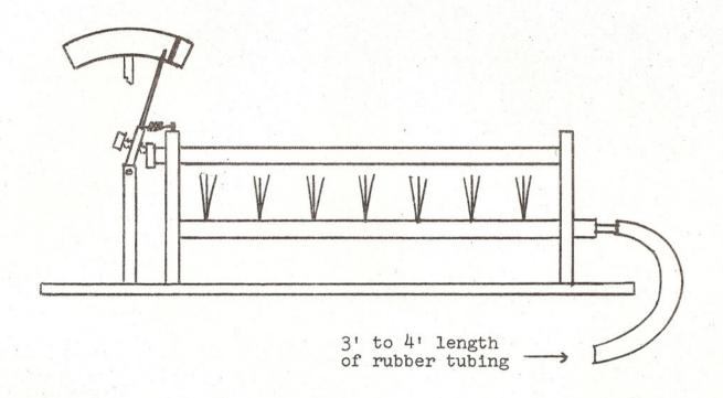
Use a long, brass tube mounted over a long, gas-fed burner. (See Note 1.) Adjust screw until pointer stands at red index mark on circular scale. Turn gas on full and light burner, moving match along entire length of burner to ignite all jets. (See Note 2.) Observe the movement of the pointer as the brass tube is heated. (See Note 3.)
