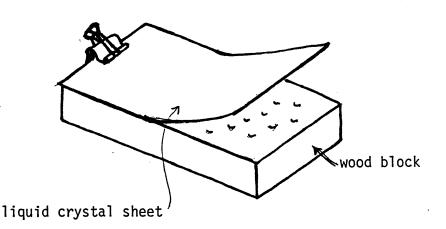
Remove the liquid crystal sheet from the apparatus, hold it up for the class to see, and touch the back of it with your fingertips to show that it changes color with the application of neat. (The order of colors is roughly that of the spectrum.)
