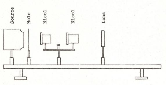
Before demonstrating the behavior of a Nicol prism, you may wish to show the wooden model and explain how the crystal is cut and recemented to form the Nicol.
