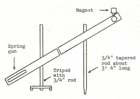
Set tapered rod in the tapered receptacle second from the (lecturer's) right, front corner of lecture table. Mount apparatus as illustrated above, at an angle of elevation about as large as possible.
