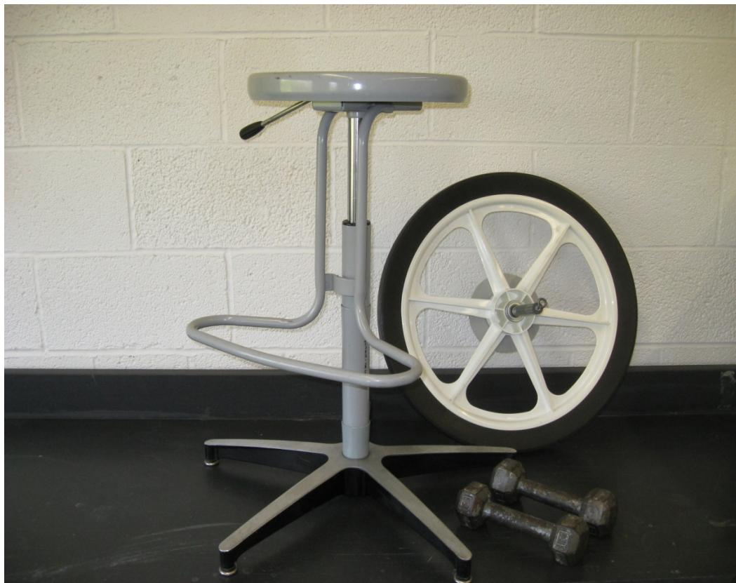
Using hand weights: Sit on stool, hold hand weights extended at arm's length, and have someone start you rotating slowly. Pull the weights in quickly; then let the weights out quickly. Making the changes quickly minimizes the effect of friction.
