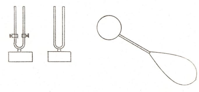
Use two identical, 256-cps tuning forks mounted on resonant boxes. Place boxes parallel, 6 to 10" apart, with open ends toward students.
